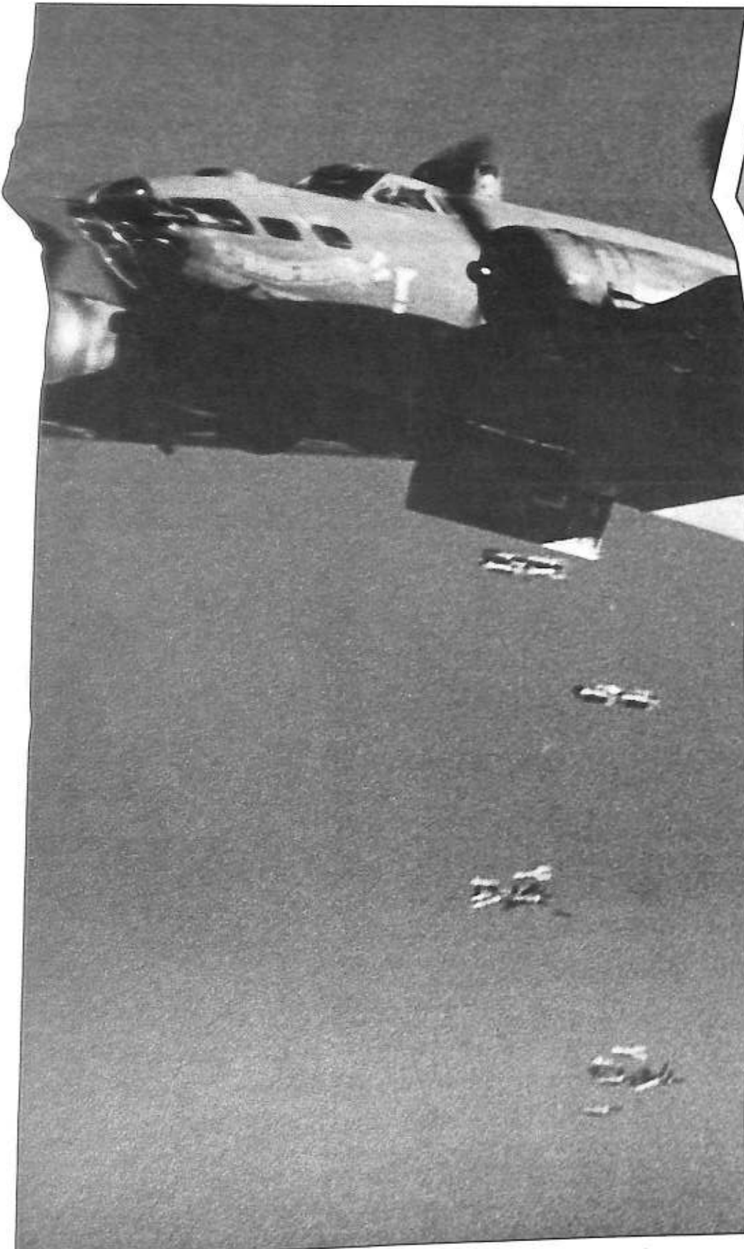
Note in this unusual picture that the plane is dropping incendiary clusters, and as they move earthward the clusters are coming apart to separate the incendiaries so that they will give broad coverage of the target area.
